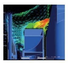
the insulation material to its limits. It also eliminates any hotspots by providing a uniform temperature distribution throughout the frame.
